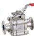
SERIES 88SN Direct Mounting Design Size: 1/2" - 4" True Tube Full Port Body/Ends: 316L S/S Ball/Stem: 316L S/S Seats: PTFE Rating: 1000 PSI max.
