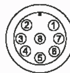
M12 Connector (8-pin) (front view)
