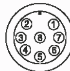
M12 Connector (8-pin) (front view)
