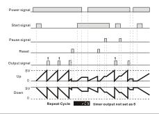
The leading edge of a "reset" input signal at RST1 will turn OFF the outputs and reset the timing period. The "reset" signal minimum pulse width is set by reset pulse width parameter ( **FE5F**). The leading edge of a new "start" signal is necessary to restart the cycle.
