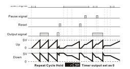
The trailing edge of the "start" signal has no effect on the outputs or timing period.
