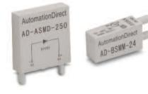
When inductive load devices (motors, motor starters, interposing relays, solenoids, valves, etc.) are controlled with relay contacts, it is recommended that a surge suppression device be connected directly across the coil of the field device. If the inductive device has plug-type connectors, the suppression device can be installed on the terminal block of the relay output.
