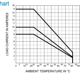
Note: A minimum spacing of 17.5 mm (0.7 in) between adjacent 861 relays is required in order to achieve the maximum ratings. A Omm spacing will result in a 50% reduction in the de-rating.
