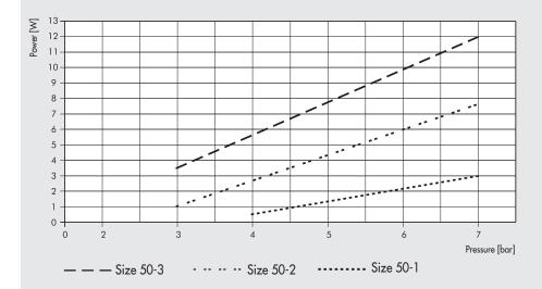
Important: if the input pressure is not sufficient to generate the power required by the electric load, the generator keeps switching on and off (intermittently). You only need to increase the air pressure (as shown in the chart) to get the required power.
