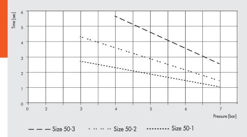
The above graph shows, for a set input pressure, the maximum time required to reach the rated output voltage (with maximum electrical load applicable for this pressure) as the size of the device changes. For example, with a size 50-2 device having an input pressure of 5.2 bar, a 24VDC output voltage will be available about two seconds after start-up.
