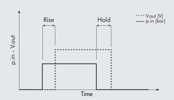
**Rise time:** the delay from activation of the compressed air supply to 24V power supply to the M8 connector.
