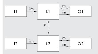
Were: im: interconnection means 11, 12: input device, e.g. sensor L1, L2: logic m: means of surveillance O1, O2: output device, e.g. valve c: crossed check
