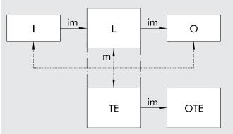
Were: im: interconnection means I: input device, e.g. sensor L: logic m: means of surveillance O: output device, e.g. valve OTE: Test Equipment OUTPUT TE: Test Equipment
