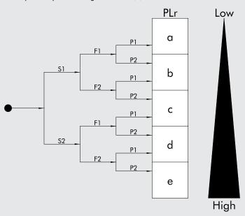
If, for example, the severity of a lesion resulting from a failure is low and/or the hazard exposure frequency is low and/or the hazard avoidance possibility is high, the PLr will be low. On the contrary, if the severity and/or exposure frequency is/are high and/or the hazard avoidance possibility is low, then the PLr for that safety function will be high.
