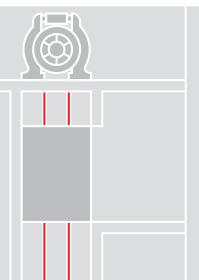
Nowadays an overspeed governor and an incremental or absolute encoder for simple and reliable shaft copy are a safety system absolutely necessary for any elevator installation.
