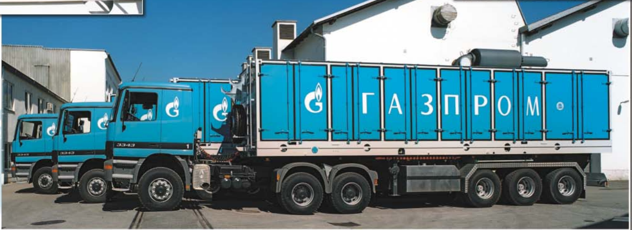
▲ Truck-mounted compressor units with HP compressor VCS-3421 W 15 delivery 67 m 3 /min (2370 cfm), working pressure 150 bar (2175 psi), driven by 16 cylinder 1.3 MW (1770 hp) diesel engine, containerized for ambient temperatures +35/-50 °C
