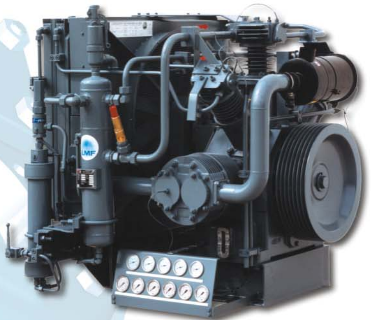
◀ V19 / 5621 L 35 delivery 4570 ltrs/min (161 cfm), working pressure 350 bar (5075 psi), driven by 110 kW (150 hp) electric motor
