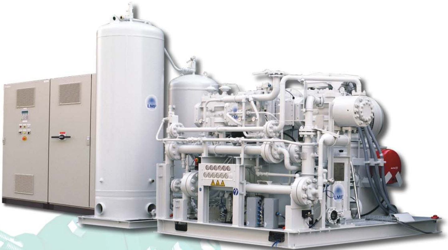
▲ LMF CNG compressor BS302 - 313 S 25/30 capacity 1254 - 2145 Nm 3 /h (780 to 1335 scfm), suction pressure 11,35 - 18,25 bara, speed 1500 rpm / 315 kW 430 hp) main drive
